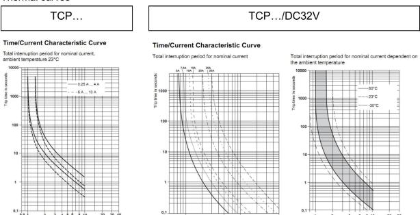
Due to the thermal inertia of the bimetallic strips, the characteristic curve slopes downward slowly. As a result, thermal circuit breakers are suitable only for overload currents and not suitable for short-circuit currents.
