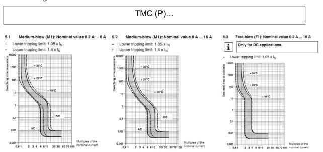
Whereas the slight decline at the top of the curve is due to the slow thermal heating of the bimetallic strips, the steep decline in the curve is caused by the magnetic short-circuit release.
