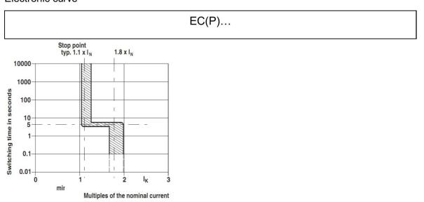
The electronically defined trigger thresholds result in a curve with very steep sides. The switch-off point begins at 1.1 x IN. If this is exceeded for more than 3-5 seconds, the device will be switched off. The current is actively limited at max.  $1.8 \times IN$ .
